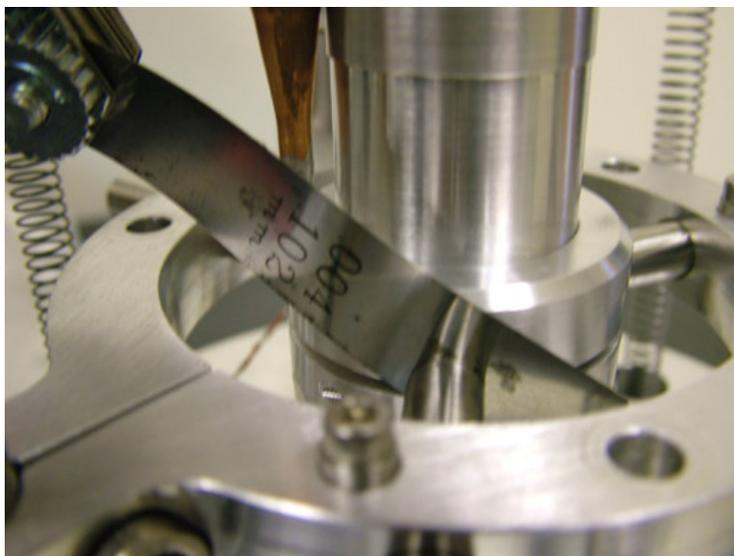
**Figure 4-3 Superspring Guide Pins And Feeler Gauge**
